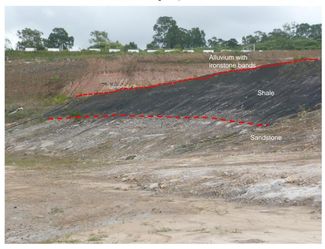
Figure 4: Photograph in Glenfield Waste Facility showing general stratigraphy looking northwest
